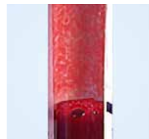
Figure 3. A correctly mixed tube.
